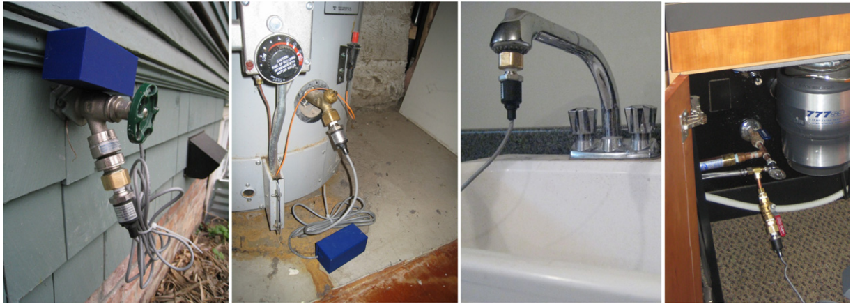
Fig. 1. HydroSense can be easily installed by screwing the pressure sensor onto an exterior hose bib, water heater drain valve, or utility sink faucet (in the same way that one would attach a garden hose). If these installation points are not available, HydroSense can also be installed at the 3/8" hose connection points of toilets, bathroom and kitchen sinks (far right image).
