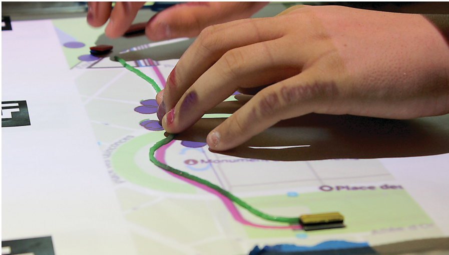
Figure 4. The VISTE project [6] ( http://visteproject.eu/ ) combines tangible user interfaces and augmented reality to make maps more accessible for users with visual impairments.
