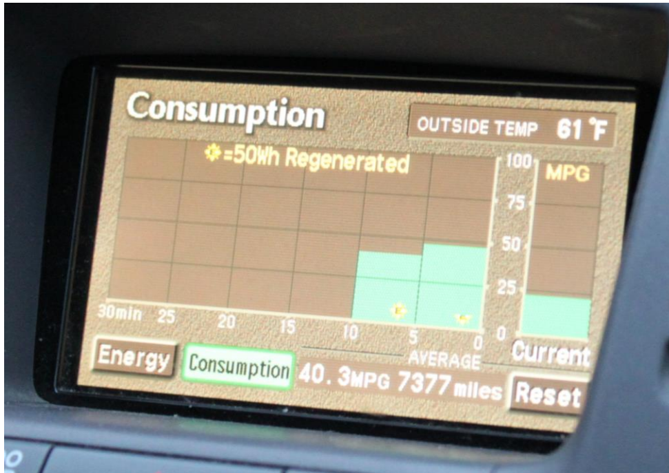
Figure 8: The original Toyota Prius eco-driving dashboard display, which includes instantaneous feedback on current fuel efficiency, a moving bar graph of average fuel efficiency in five minute intervals overall the last 30 minutes, the overall fuel efficiency since the trip odometer was last reset, and a “40Wh Regenerated” badge icon for regenerating energy via braking.
