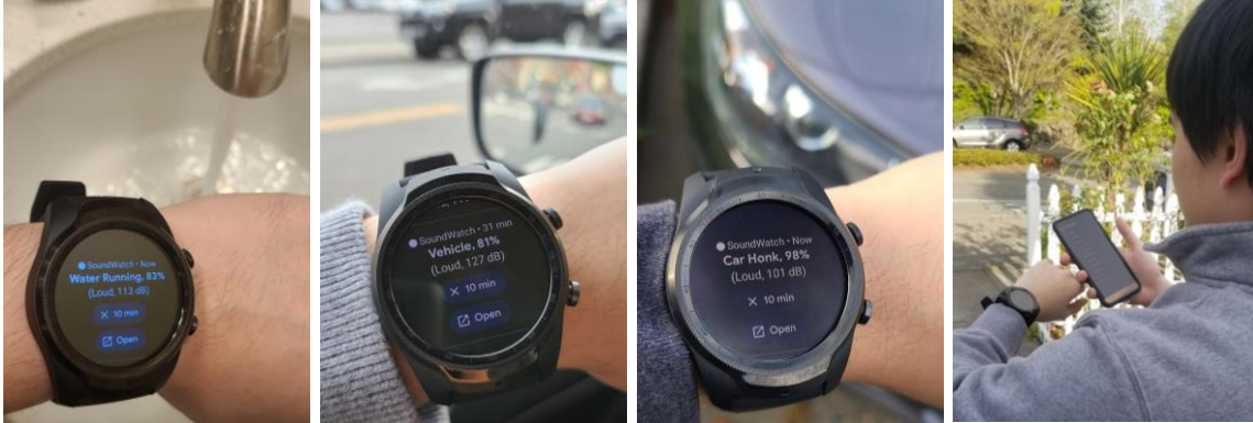
Figure 4.1: SoundWatch uses a deep-CNN based sound classifier to classify and provide feedback about environmental sounds on a smartwatch in real-time . Images show different use cases of the app and one of the four architectures we built ( watch+phone ).
