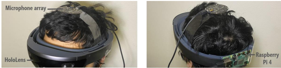
Figure 6.12: The three components of HoloSound system.
