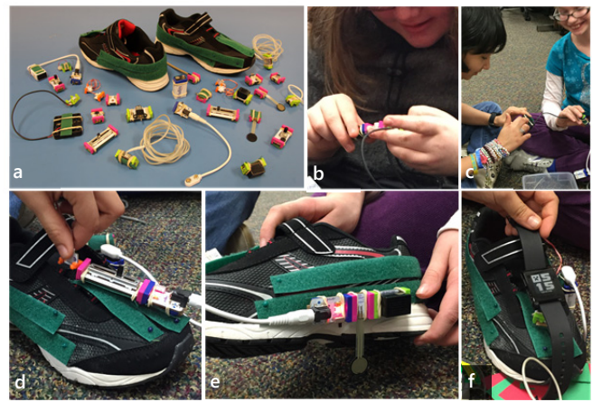
Figure 3: In the second CI session, two co-design teams were provided with littleBits and shoes (a) modified with Velcro for attachment. Teams first examined and played with littleBits to build up understanding (b-c) before designing their own littleBits-based MakerShoes (d-e). In the last co-design activity (f), teams could create new functionality using everyday objects (e.g., a watch) and cardboard (red for input, green for output).
