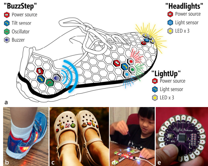
Figure 1: MakerShoe is an e-textile construction kit aimed at engaging young children (K-4) in wearable design. (a) Using only a few modules, this MakerShoe buzzes and lights up during movement and turns on ‘headlights’ when it’s dark. The bottom row highlights a few inspirations including: (b) traditional light-up shoes, which are fanciful, fun, and responsive but not modifiable; (c) self-expression through fashion personalization (e.g., Crocs Jibbitz shoe charms); (d) littleBits electronic construction kit [1]; (e) and the LilyPad e-textile Arduino [3].
