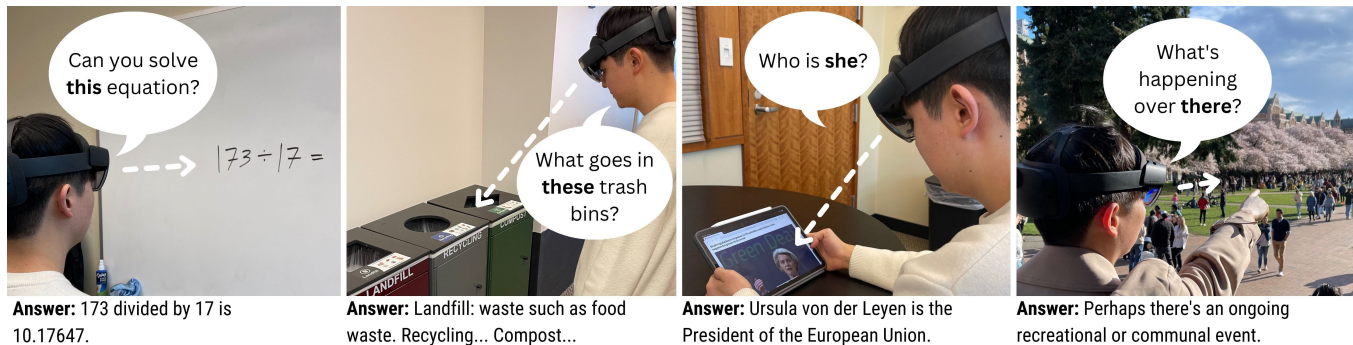
Figure 1: Example interactions with GazePointAR. Pronouns such as “this,” “these,” “she,” and “there” are automatically resolved by using real-time gaze tracking, pointing gesture recognition, and computer vision. See demo video for interactive examples.
