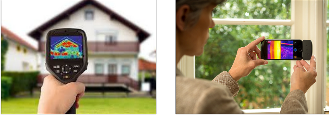
Figure 1.1: Thermal cameras come in many form factors including handheld models (left) and more recently released smartphone-based thermal camera attachment (right); images courtesy of the DOE website [146].
