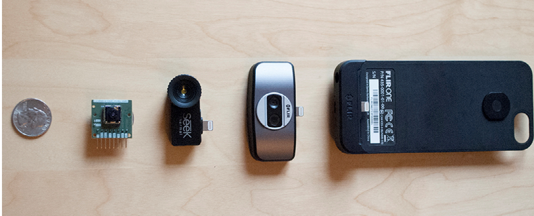
Figure 2.1: Commodity thermal cameras for smartphones and small electronics projects. From left to right: FLIR Breakout Board, Seek Thermal Imaging Camera for iOS, FLIR One iOS Attachment Gen II, FLIR One iOS Attachment Gen I.
