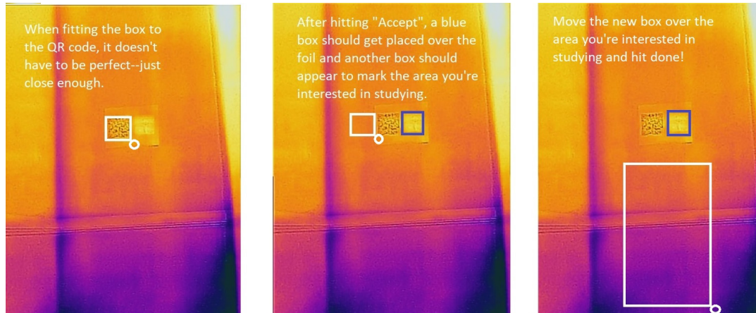
Figure 7.3: Calibration Procedure. After receiving the inferred emissivity map a box appears over the QR code or in the middle of the screen if the QR code was not found (left); by dragging the white box users can update the position and by dragging the small circle users can resize it. When the user accepts the QR code position using on screen buttons (not shown) the distance to the wall and the position of the high-emissivity foil is inferred (middle). A second box appears on screen to the left of the QR code (middle); the user can move the second white box to select the region they are interested in scanning (right). When users select ‘Done’ the calibration is complete.
