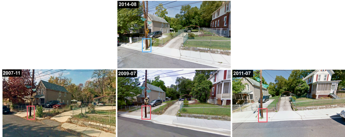
Figure 4-2: Framework results for “Objects in path” category. The blue label refers to the manually labeled ROI on the most recent snapshot (input of the framework), and red labels are localized by the framework, referring to the existence of accessibility problems on all previous snapshots.
