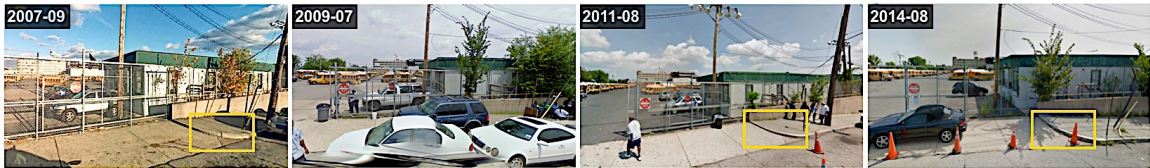
Figure 3-11: Tracking the missing curb-ramps in a location, where the curb is occluded in one of the snapshots (2009-07). However, the curb still exists in 2011-08, meaning that the occluded snapshot can be ignored.
