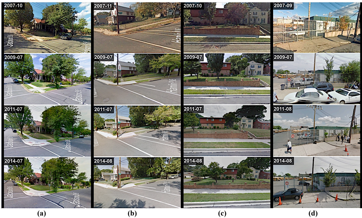
Figure 3-2: Examples of locations with various transitions in terms of accessibility features: (a) the missing curb-ramps changed to accessible curb-ramps, (b) the missing curb-ramps still exist, (c) the sidewalk remains accessible, (d) vehicles obstruct the view of missing curb-ramps in 2009-07.
