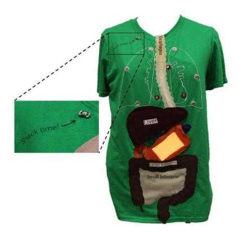
Figure 33: The "snack time" button triggers the digestive system shown here. stomach and embedded LEDs in the remaining digestive system organs. The visualization begins with a push of the "Snack time!" button (Figure 33). The esophagus, which consists of a Neopixel LED strip covered with fabric, lights up to illustrate the movement of food traveling down (Figure 34).
