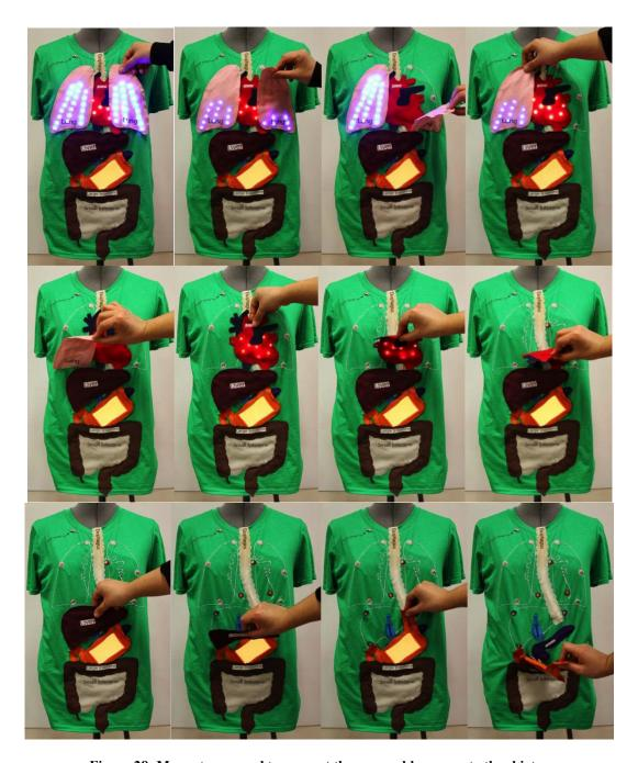
Figure 28: Magnets are used to connect the removable organs to the shirt. When detaching the removable organs from the shirt it is sometimes difficult to identify where they must be reattached. I produced two designs to address this issue. First, I placed color-coded "highlighters" around each wire spiral on the shirt to guide reattachment of organs (Figure 27). These highlighters are small fabric circles
