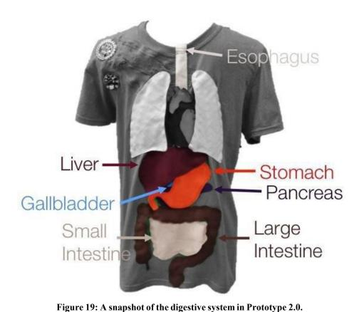
The digestive system was created without functionality in this prototype due to time constraints towards the second Kidsteam session and additional flaws discovered when using conductive thread. These flaws were revised in Prototype 2.1, described later in this Chapter.
