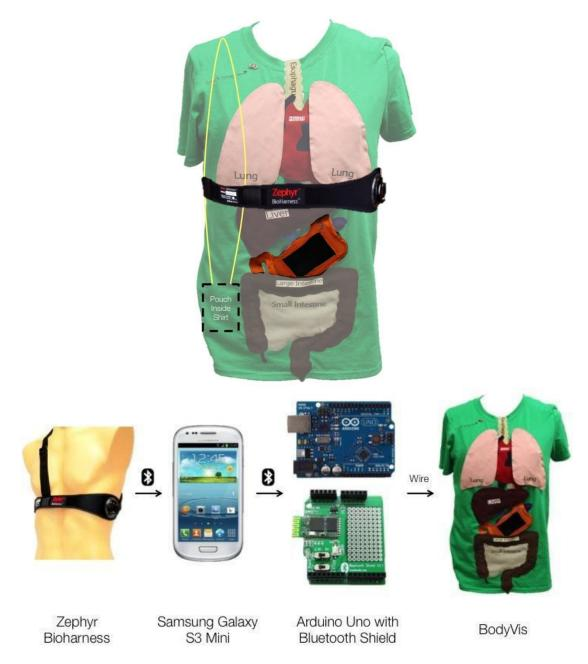
Figure 32: The Bioharness (shown on top of shirt for clarity), Android phone (Galaxy S3 Mini), and Arduino (in pouch) are embedded into the shirt (on top). The Bioharness sends bio-data to the Android phone via Bluetooth; the phone translates this data and sends it to the Arduino via Bluetooth; the Arduino is wired to and controls the LEDs in the organs (on bottom).
