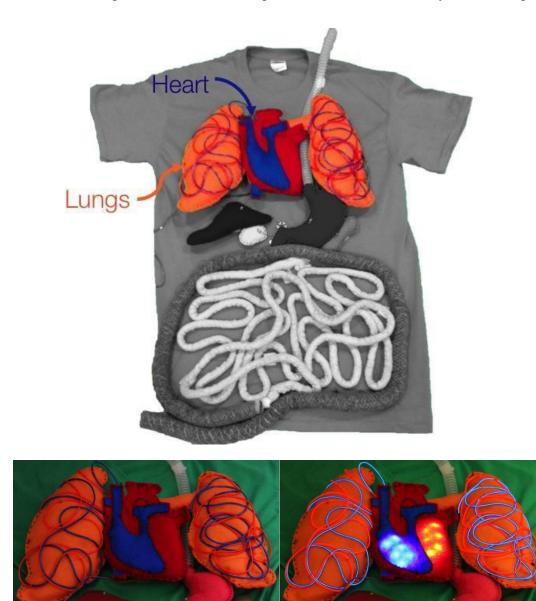
Figure 10: On top, the heart and lungs in Prototype 1. On bottom, a close-up of the fabric heart (red and blue) with embedded LEDs and lungs (orange) with vein accents made of EL wire.
