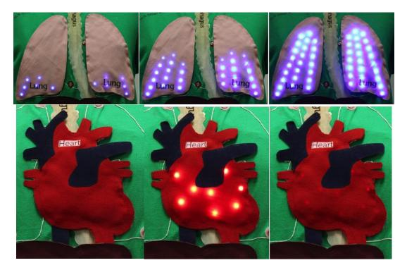
Figure 31: Lungs "inflate" when the LEDs fade on upwards (top left to right), and vice versa when they "deflate." The LEDs in the heart abruptly turn on and fade off to mimic a heartbeat (bottom left to right).
