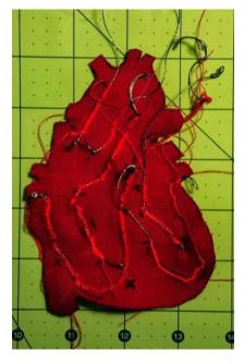
Figure 17: The heart contains LED pixels connected by conductive thread (silver thread), held down and protected by nonconductive thread (red thread).
