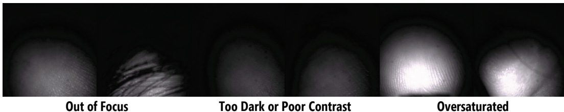
Figure 7.4: Approximately 5% of the images we collected had poor focus, contrast, or illumination, preventing robust feature extraction. We adjusted the camera and LED to mitigate these issues for TouchCam Realtime.
