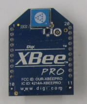
xbee wireless modem
