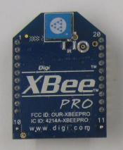
xbee wireless modem
