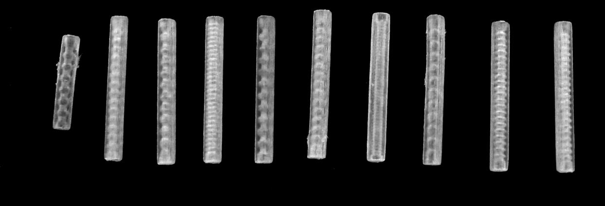
Major factors that contributes the generation of distinct pulses: Tube length, tube diameter, corrugation shape, corrugation gap, and the geometry of corrugation
